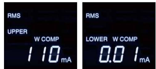
▲AC Hipot (Withstanding voltage) test settings display (example)
