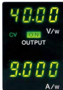
\* The maximum number of digits displayed on the ammeter (i.e. the location of the decimal point) varies according to the model.
